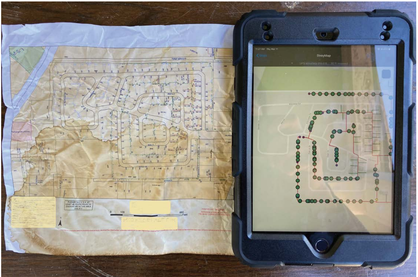
FIGURE 5 —DAMAGED PAPER AS-BUILT MAPS CAN BE EASILY DIGITIZED AND ADDED TO ONLINE AND MOBILE DEVICES FOR LIVE UPDATING
