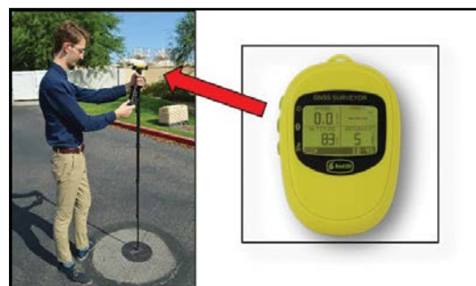
FIGURE 16—BAD ELF GNSS SURVEYOR UNIT AND AN EXAMPLE OF HOW IT IS USED IN THE FIELD 9
