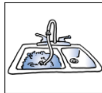
Putting the garden hose down the drain to flush out debris when it's backed up.
